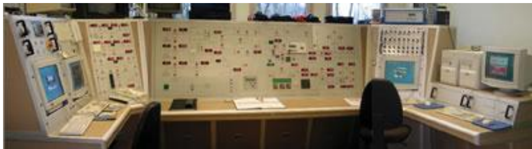
Figure 3. Bench control. Control computers and bench front end electronics at MASCOTTE test bench premises at Onera (Palaiseau, France).
